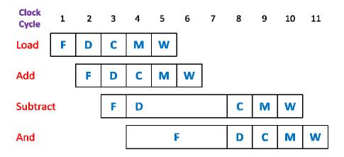
(c) (6 points) Now, assume that the pipeline <u>uses</u> operand forwarding. There are separate forwarding paths from the outputs of stage-3 and stage-4 to the input of stage-3. Draw a diagram that represents the flow of instructions through the pipeline during each clock cycle. Indicate operand forwarding by arrows.
